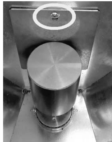
Fig. 38 - Remove the screw
