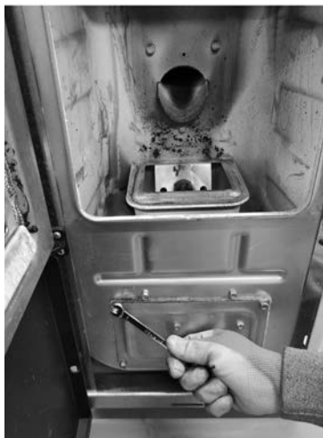
Fig. 29 - Remove the screws
