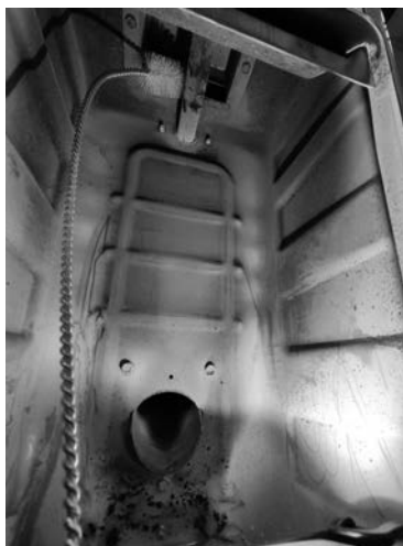
Fig. 33 - Clean with pipe cleaner
