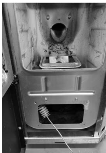
Fig. 31 - Clean with pipe cleaner
