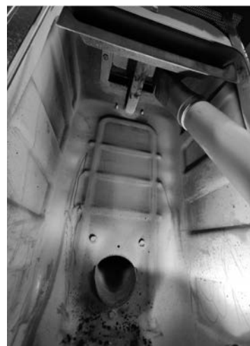
Fig. 34 - Vacuum out the ash
