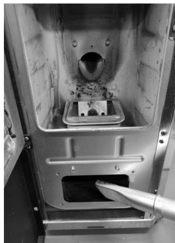
Fig. 32 - Vacuum out the ash
