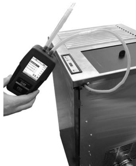
Fig. 27 - Digital pressure switch connection
