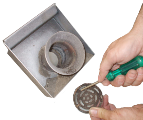
Fig. 36 - Burning pot cleaning
