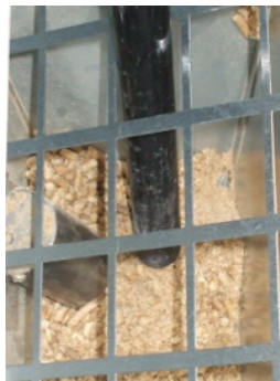
Fig. 40 - Hopper and auger cleaning
