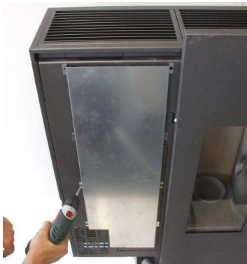
Fig. 41 - Heat protection panel removing
