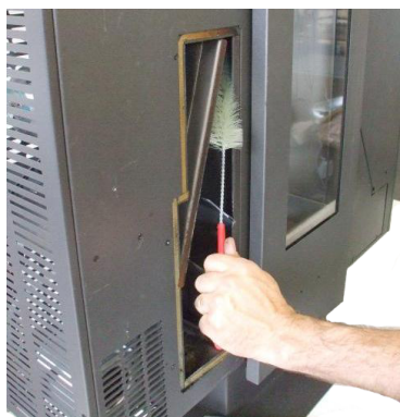
Fig. 43 - Cleaning with a brush
