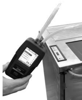
Fig. 61 - Digital pressure switch connection
