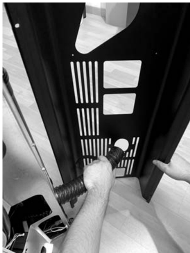
Fig. 56 - Feeding flexible hose 2
