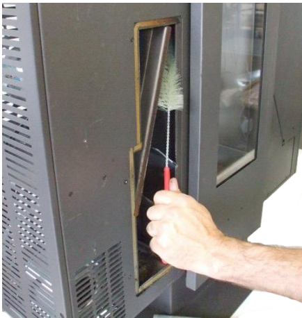
Fig. 44 - Cleaning with a brush
