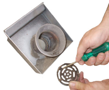
Fig. 38 - Burning pot cleaning
