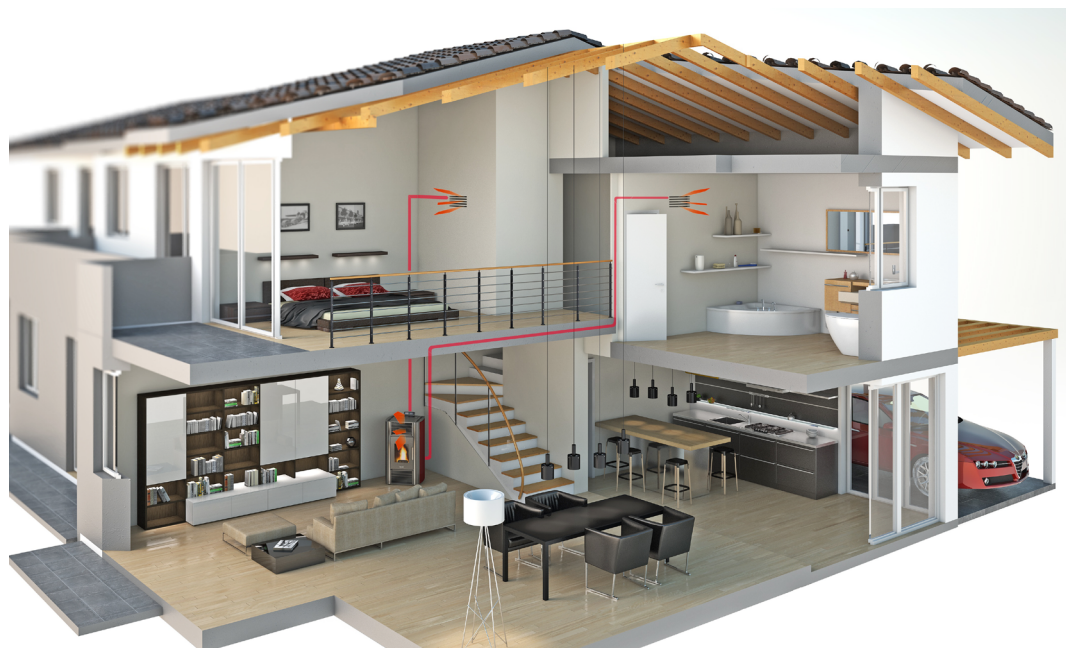
Fig. 31 - Ducting system example
