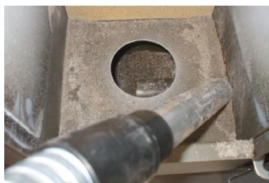
Fig. 39 - Ash tray box cleaning
