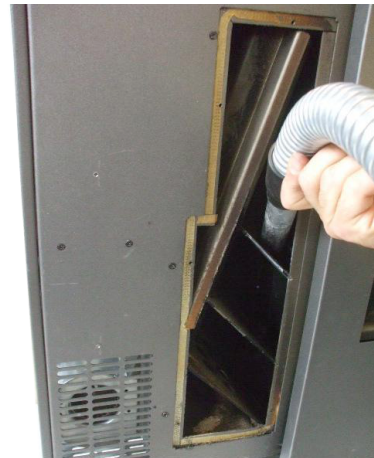
Fig. 45 - Fume chamber cleaning
