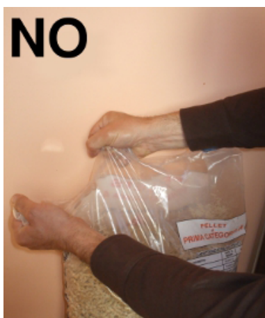
Fig. 34 - Wrong opening of the pellets bag
