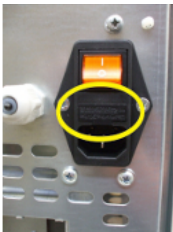
Fig. 51 - Shutter with the fuse to remove
