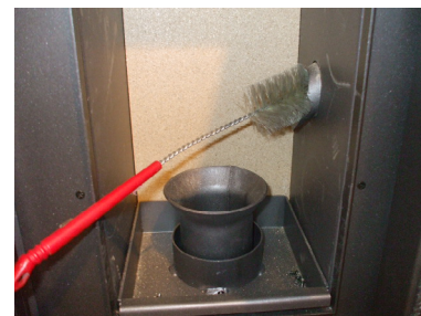
Fig. 41 - Cleaning with a brush
