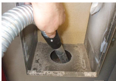
Fig. 40 - Burning pot box cleaning
