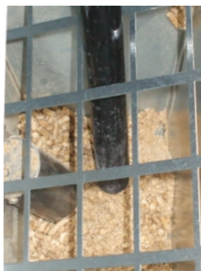
Fig. 39 - Hopper and auger cleaning
