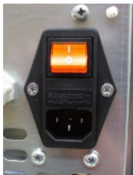
Fig. 26 - Electric socket with master switch
