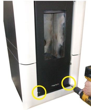
Fig. 22 - Frontal panel position
