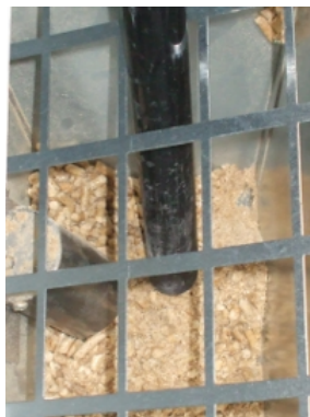
Fig. 36 - Hopper and auger cleaning
