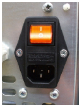
Fig. 24 - Electric socket with master switch
