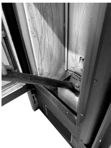
Fig. 29 - Burning pot box cleaning
