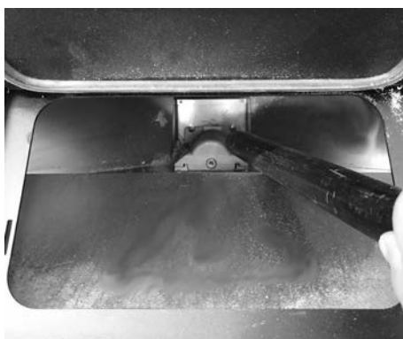
Fig. 31 - Hopper cleaning
