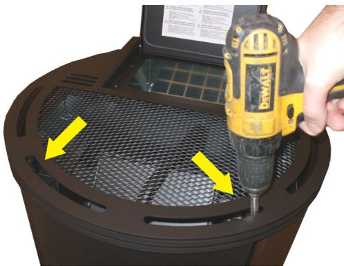
Fig. 67 - Cover 1 screw removal
