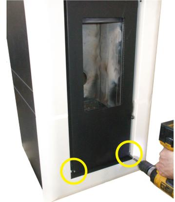
**Fig. 38 - Frontal panel fixing**
