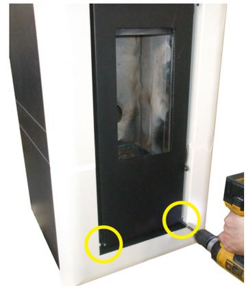
**Fig. 24 - Frontal panel fixing**
