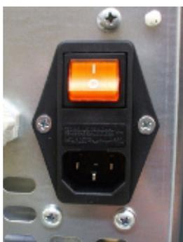
**Fig. 43 - Electric socket with master switch**
