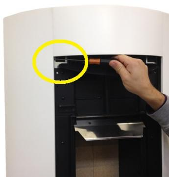
Fig. 73 - Loosen the top screw
