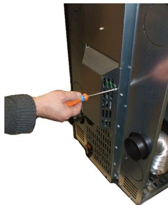
**Fig. 89 - Rear panel removal**
