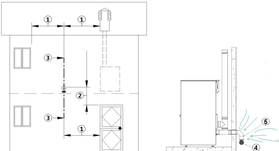
Fig. 8 - Air inlet for sealed-chamber installation
