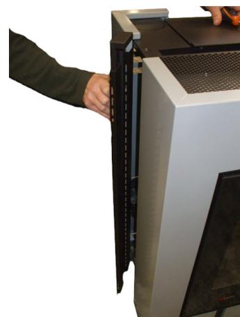
Fig. 65 - Removing the central panel
