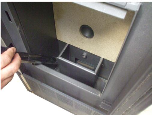
Fig. 58 - Burning pot box cleaning
