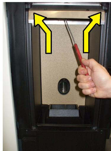
Fig. 78 - Clean both the ducts
