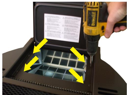
Fig. 68 - Cover 2 screw removal
