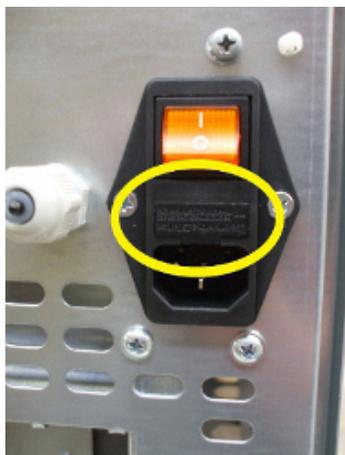
**Fig. 88 - Shutter with fuses to remove**
