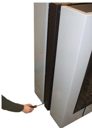
Fig. 64 - Removing the lower screws
