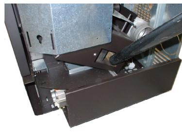
Fig. 81 - Fume chamber cleaning
