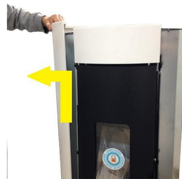
Fig. 75 - Remove side panels
