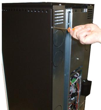
Fig. 62 - Removing the rear screw
