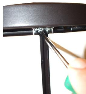
Fig. 32 - Screw the bracket
