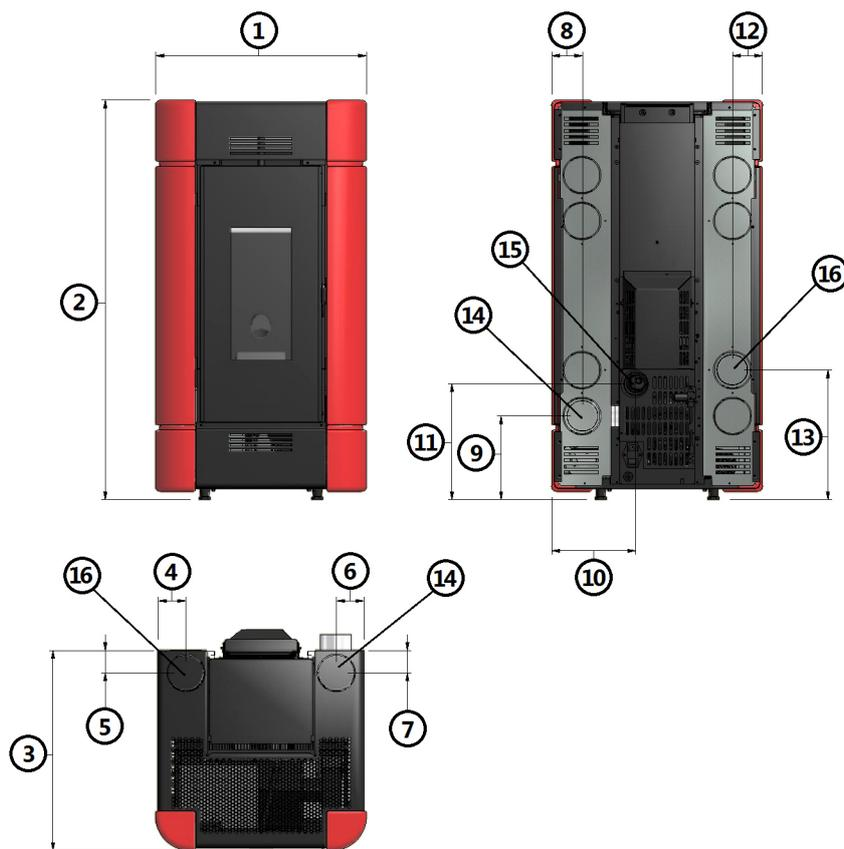
**Fig. 16 - General dimensions: Sire<sup>3</sup> Plus****LEGEND Fig. 16 page 15**
