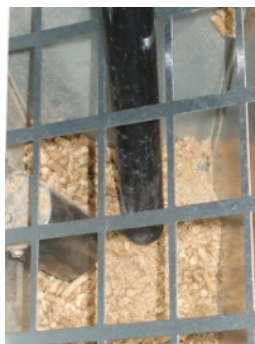
Fig. 33 - Hopper and auger cleaning
