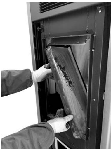
Fig. 99 - Remover as paredes laterais
