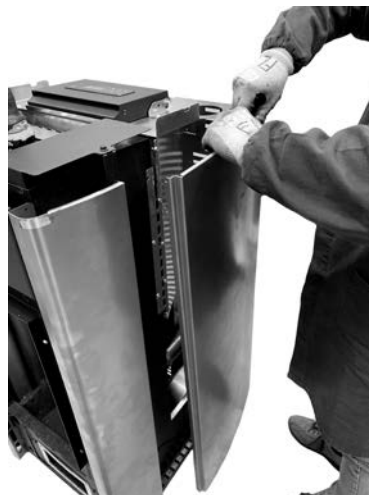
Fig. 29 - Remover as partes laterais
