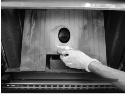
Fig. 39 - Central cast iron removal
