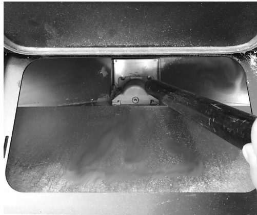
Fig. 35 - Hopper and auger cleaning
