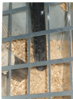
Fig. 27 - Hopper and auger cleaning
