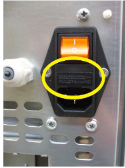
Fig. 35 - Shutter with the fuse to remove
