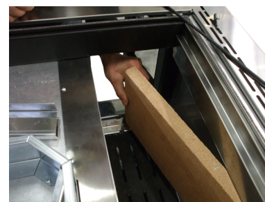
Fig. 20 - Remove the refractory material
