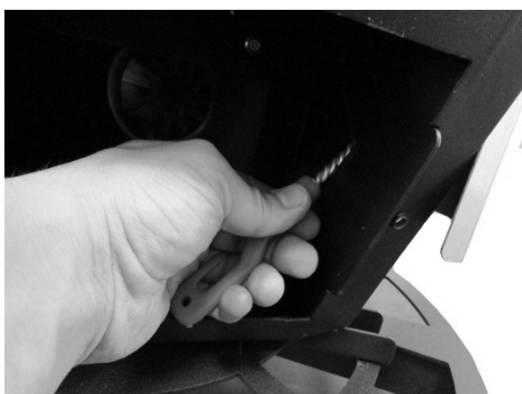
Fig. 43 - Cleaning with pipe cleaner 3
