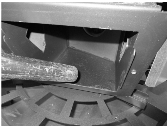
Fig. 39 - Vacuum out the ash
