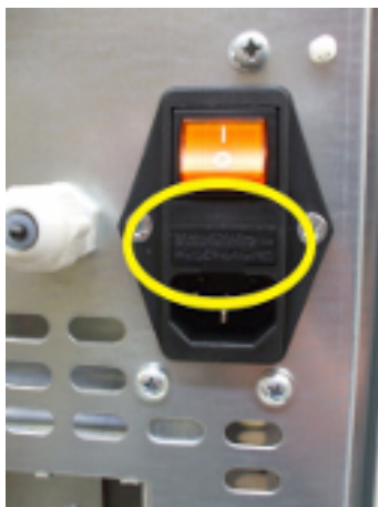
Fig. 62 - Shutter with the fuse to remove
