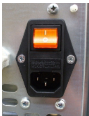
Fig. 29 - Electric socket with master switch
