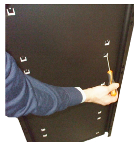
Fig. 28 - Supports to bend
