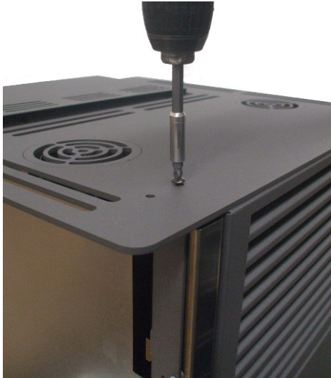
Fig. 19 - Upper screws removal
