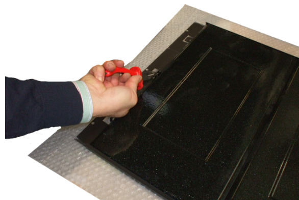
Fig. 25 - Attach the tiles
