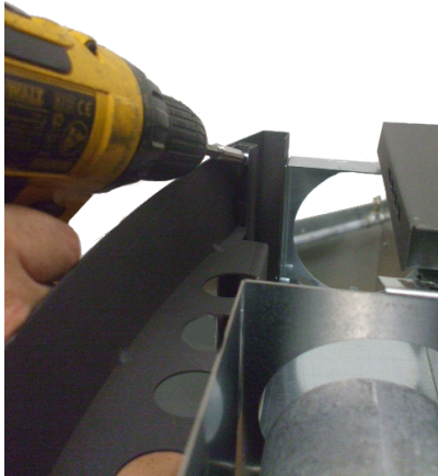
Fig. 15 - Upper curved profiles removal
