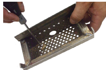
Fig. 42 - Burning pot cleaning
