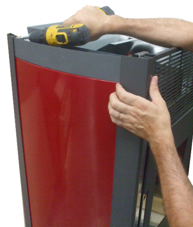
Fig. 18 - Replace upper curved profiles
