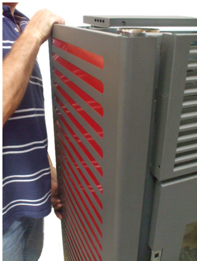
Fig. 23 - Lock the side
