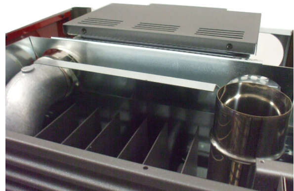
Fig. 34 - Rear ducting system
