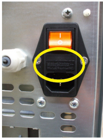
Fig. 42 - Shutter with fuses to remove
