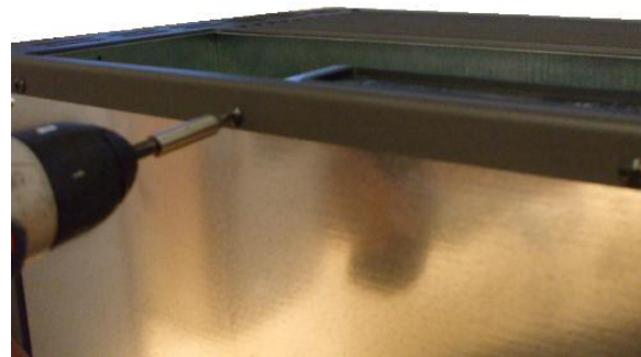
Fig. 15 - Backward screws removal
